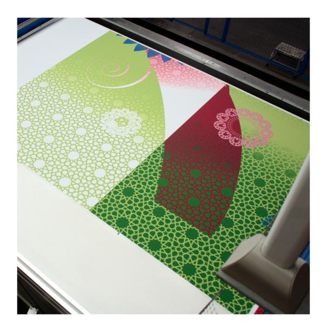
We are able to produce designs in an endless variety with only four primary colours in a digital process with our 4-meter wide Colaris and Chromojet printers. The printed colour penetrates all the way to the base, meaning high durability and minimum wear and tear.
