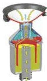
The **LAUFEN lema** 0-litre urinal saves water and money. It operates without water and does not require a water shut-off device or electricity to keep the drain closed. The urine itself helps to keep gases sealed in and to prevent their escape. The principle behind this “trap” is known in the chemical industry as the Erlenmeyer flask.
