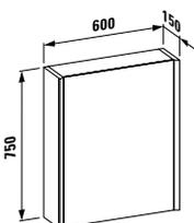
Mirror cabinet, aluminium, 2 double mirrored doors, with sensor circuit and with 2 LED lighting elements 4000 Kelvin, dimmable
