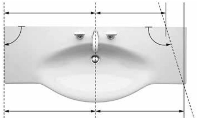
The large palace washbasins (from a length of 120 cm) can be ordered made-to-measure from our factory. Thanks to our innovative production engineering, our sanitary ware fits precisely into bathroom plans. The sanitary ware can be cut, also diagonally. Freestanding side components can also be manufactured to precise measurements without having to add on side panels with visible joints.
