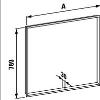
Mirror cabinet, aluminium, 1 double mirrored door, with sensor circuit and with 2 LED lighting elements 4000 Kelvin, dimmable
