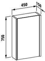
Mirror cabinet, aluminium, 2 double mirrored doors, with sensor circuit and with 2 LED lighting elements, 4000 Kelvin, dimmable
