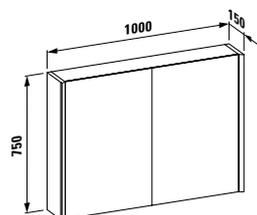
Mirror cabinet, aluminium, 3 double mirrored doors, with sensor circuit and with 4 LED lighting elements 4000 Kelvin, dimmable
