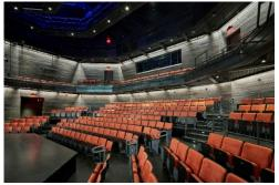
Plans were drawn up to marry perfect acoustics, flawless sightlines with custom made seating, and a reconfigured layout. Kirwin & Simpson developed a derivative of their Fleet Range suitable for the 368 Balcony, Circle and Stalls chairs. In total, 37 seats were removable and a further 2 were fitted with transfer arms for wheelchair spaces. Wall and floor mounted usher seats and portable loose chairs for use in the upper
